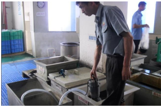
用应急泵将废液抽到应急桶
