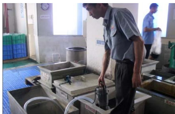
用应急泵将废液抽到应急桶
